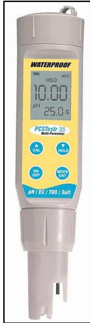
Figure 12. Waterproof Multiparameter PCS Testr 35 manufactured by Oakton Instruments ( http://www.4oakton.com ). This field instrument was used to measure various water quality parameters at each gauging station.
