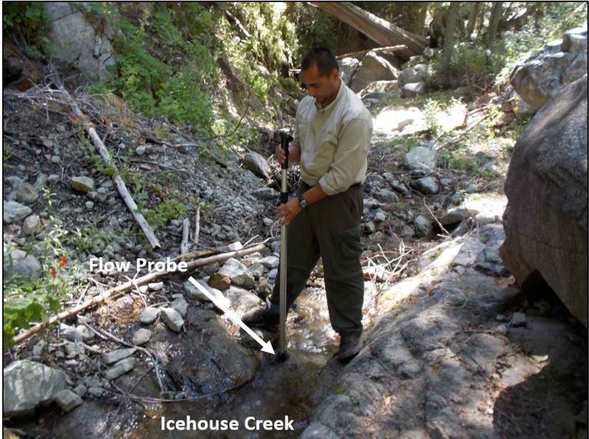
Figure 6. Measuring average stream velocity at the Broullard gauging station using a Global Water digital flow probe.
