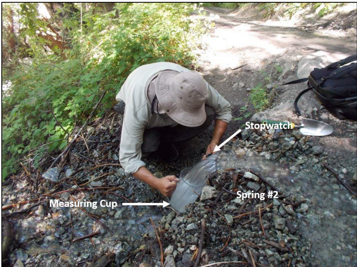
Figure 5. Capturing spring discharge using a measuring cup and stopwatch to record elapsed time.
