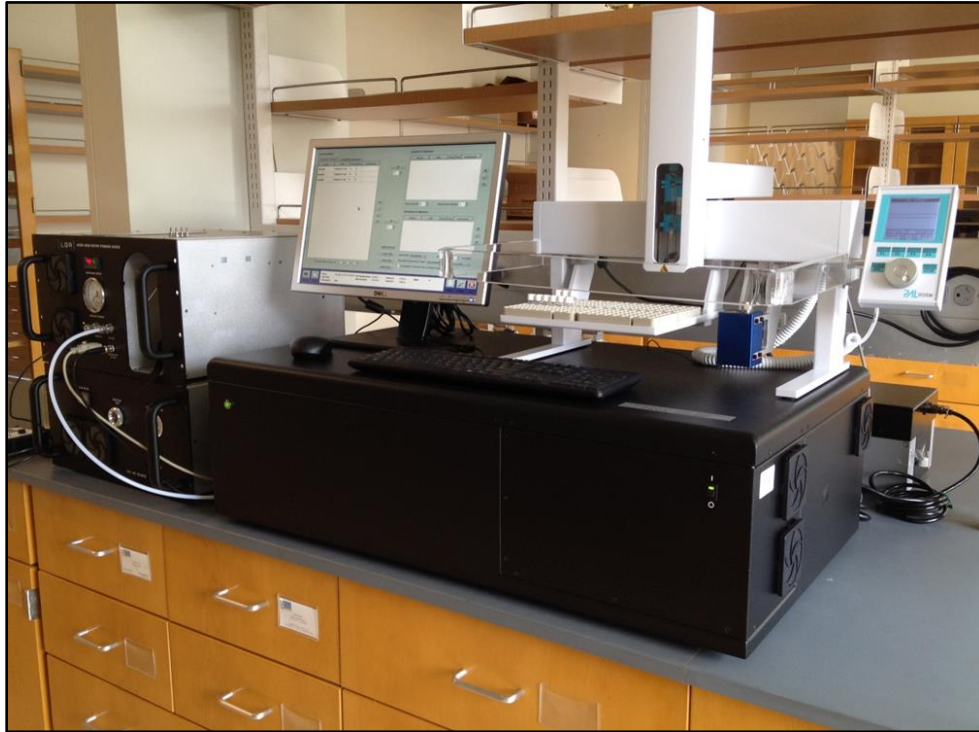
Figure 11. Laboratory equipment used to measure isotopic ratios of stable Hydrogen and Oxygen isotopes located within the Environmental Sciences Department at UC Riverside.
