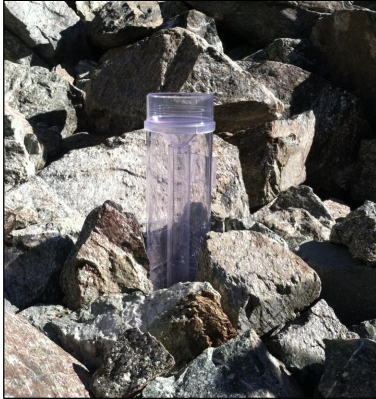
Figure 10. Photograph of an all-weather rain gauge installed at the Cabin 5 location.
