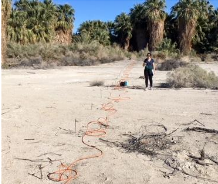
Figure 24: Resistivity survey conducted adjacent to the western margin of San Andreas Oasis. Switcher cable (orange) oriented along electrodes, with Syscal Kid control unit to the right of the line.
