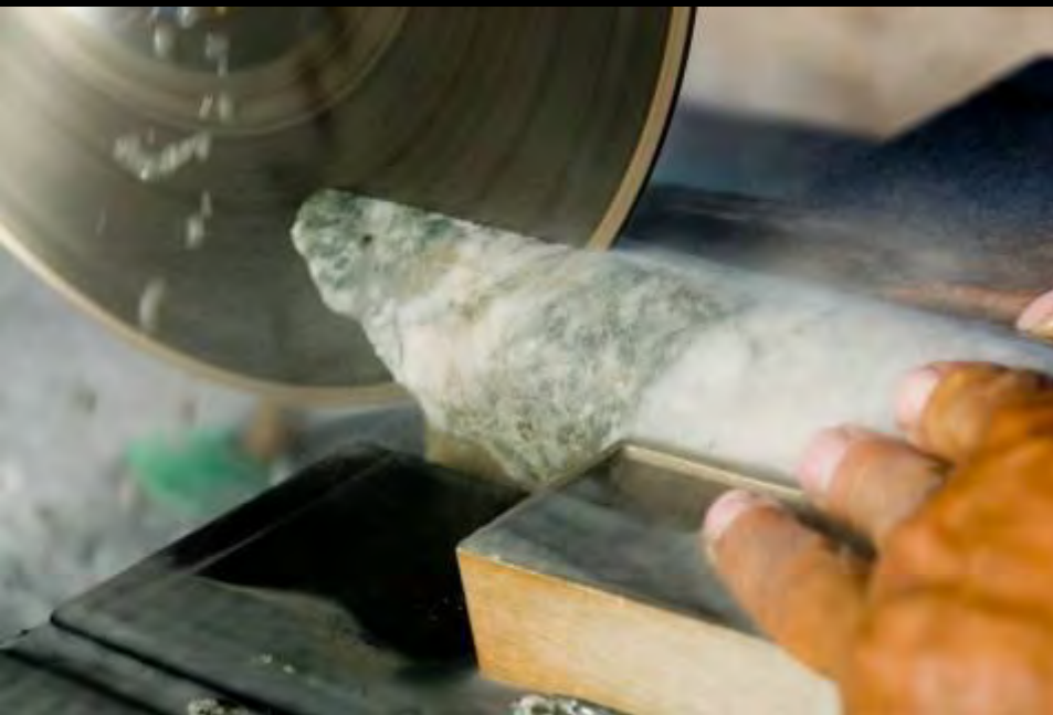
Sawing the core
