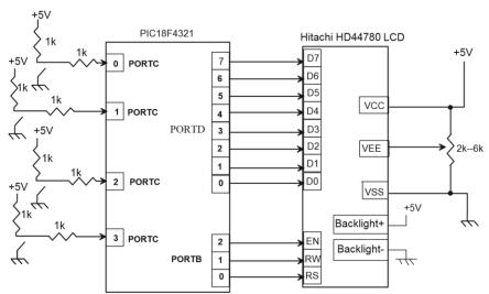
Assume the PIC18F4321- Hitachi HD44780 interface of the above figure. It is desired to display the phrase "PIC18F" on the LCD as soon as the four input switches connected to PORT C are all HIGH.
