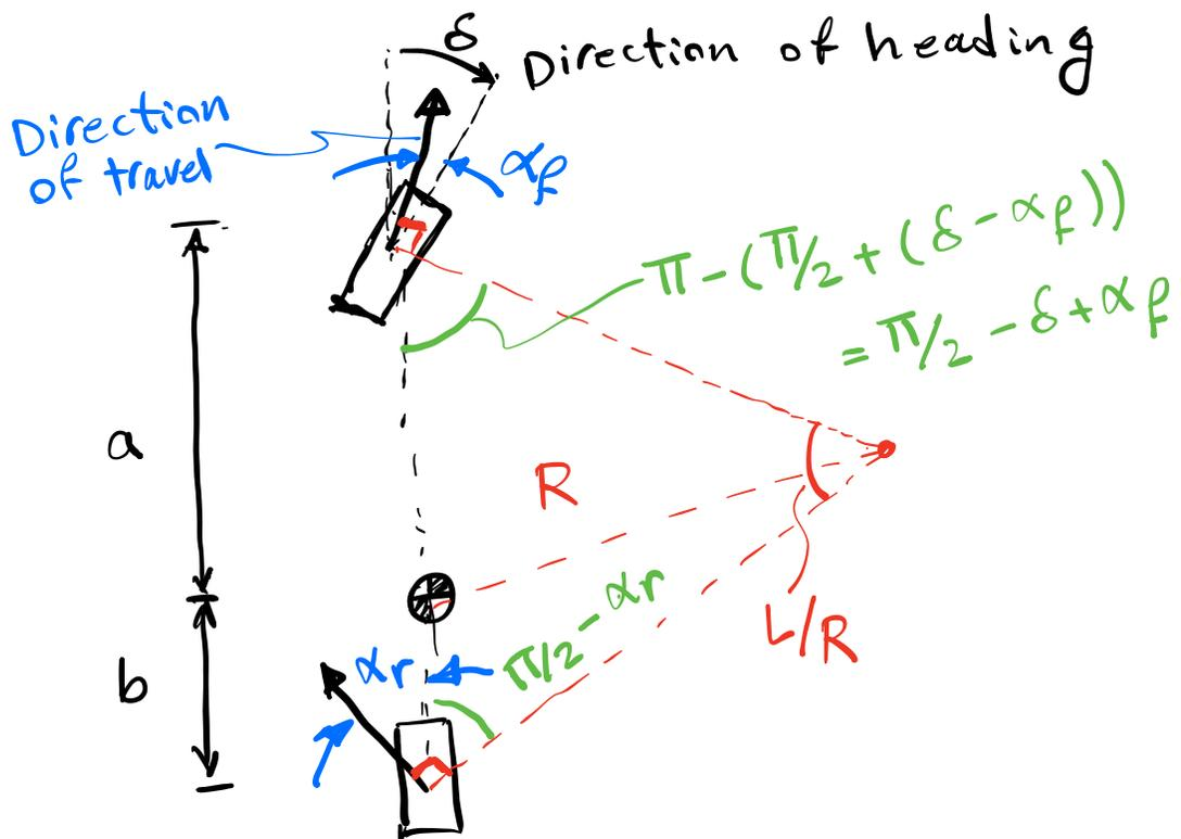
Cornering force (for low slip angles (5 degrees or less) is (the relation is linear)
