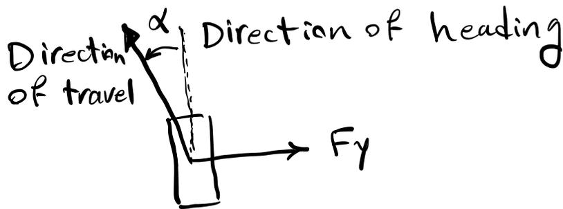
For analysis, it is convenient to represent the vehicle by the bicycle model as shown below.
