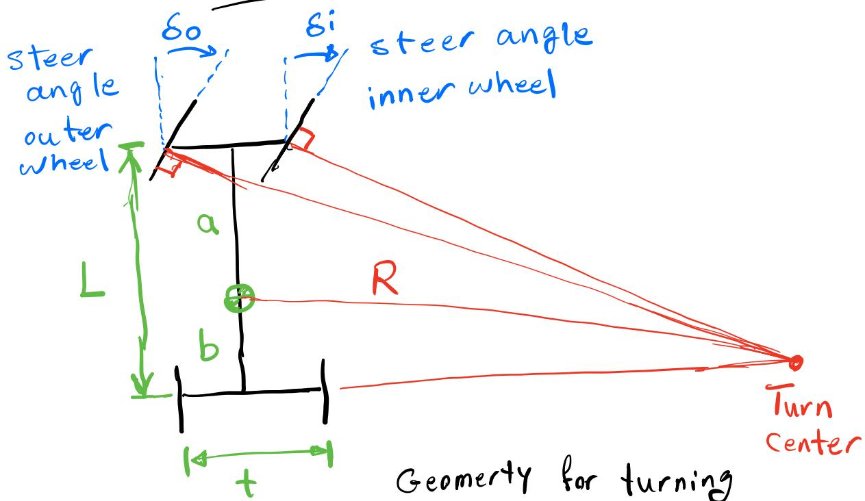
For the front wheels not to slip, they must have perpendiculars that pass through the turn center.
