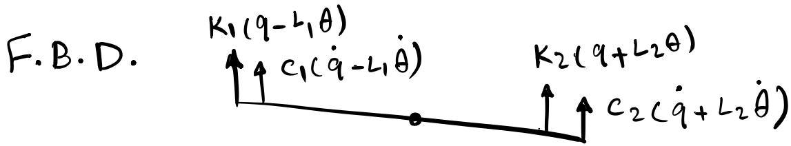
$$m\ddot{q} + c_1(\dot{q} + L_1 \dot{\theta}) + c_2(\dot{q} + L_2 \dot{\theta}) + K_1(q - L_1 \theta)$$
