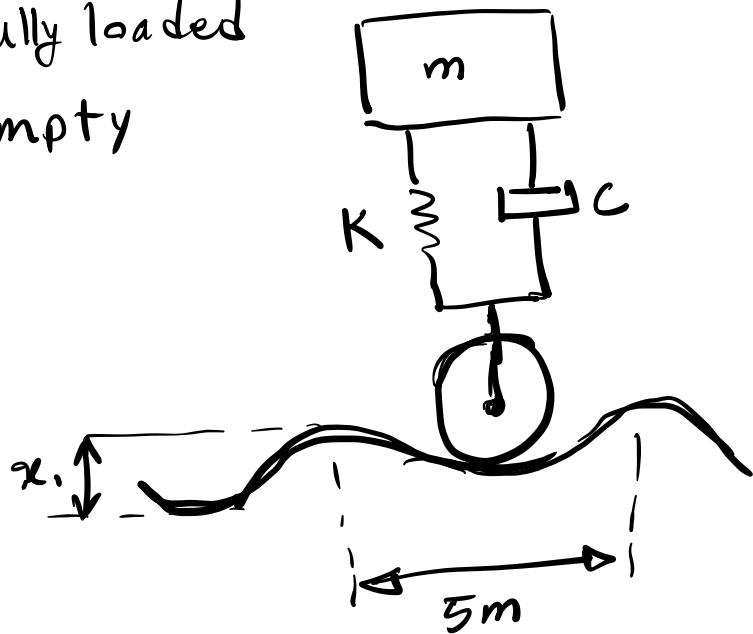
Determine the amplitude ratio of the vehicle when fully loaded and empty.
