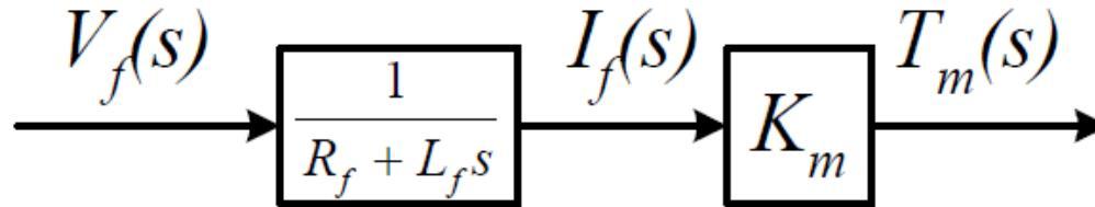
The load:  $T_m(t) - B\omega(t) = J \frac{d\omega(t)}{dt}$   $\xrightarrow{\mathcal{L}}$
