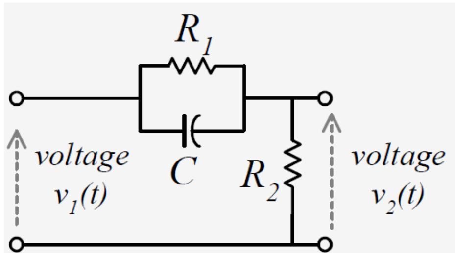
$$G_N(s) = \frac{V_2}{V_1} = \frac{R_2}{R_2 + \frac{R_1 \frac{1}{Cs}}{R_1 + \frac{1}{Cs}}} \\ = \frac{R_2}{R_1 + R_2} \frac{(1 + R_1 Cs)}{1 + \frac{R_1 R_2 C}{R_1 + R_2} s}$$
