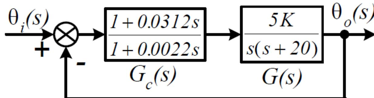
A compensator (controller) is inserted into the forward path of the system in order to improve control performance.
