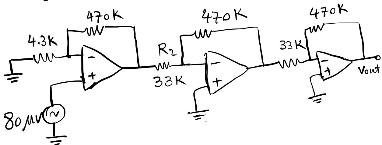
$$V_{out} = \left(1 + \frac{470}{4.3}\right) \left(-\frac{470}{33}\right) \left(-\frac{470}{33}\right) 80 \mu V$$
