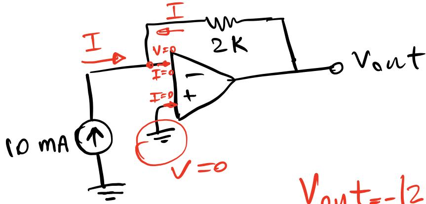
$$V_{out} = -(2 \text{ k})(10 \text{ mA})$$
