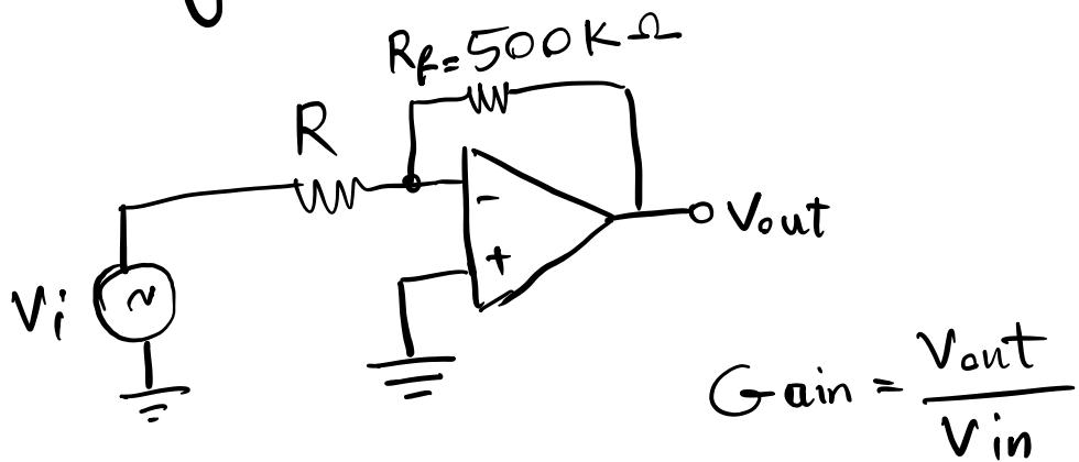
$$\frac{V_{out}}{R_f} = -\frac{V_i}{R} \Rightarrow \text{Gain} = -\frac{R_f}{R}$$
