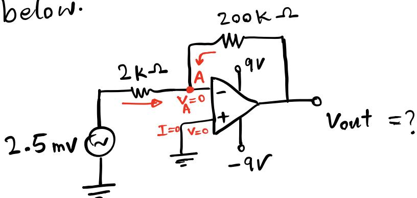
$$\frac{V_{out}}{200 \text{ k}\Omega} = -\frac{2.5 \text{ mV}}{2 \text{ k}\Omega}$$
