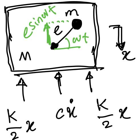
$$(M-m)\ddot{x} + m \frac{d^2}{dt^2}(x + e \sin \omega t) = -Kx - c\dot{x}$$
