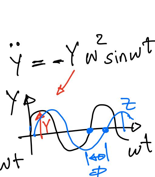
$$m \ddot{z} + c \dot{z} + K z = m \omega^2 Y \sin \omega t$$
