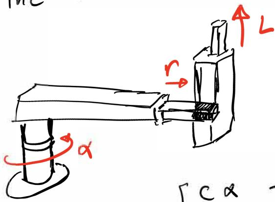
$$T_{\text{cyl}}(r, \alpha, L) = \begin{bmatrix} c\alpha & -s\alpha & 0 & r c\alpha \\ s\alpha & c\alpha & 0 & r s\alpha \\ 0 & 0 & 1 & L \\ 0 & 0 & 0 & 1 \end{bmatrix}$$
