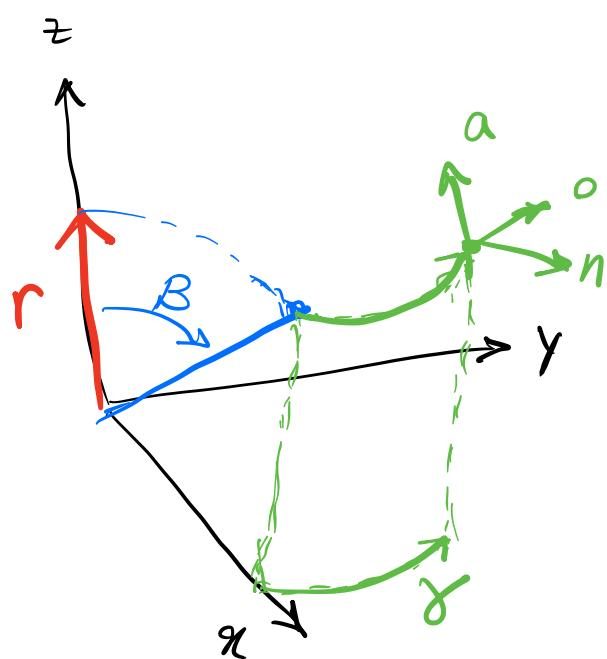
$${}^R_T P = T_{Sph}(r, \beta, \gamma) \\ = \text{Rot}(z, \gamma) \text{Rot}(y, \beta) \text{Trans}(0, 0, r)$$
