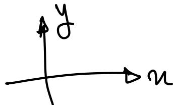
$$\left\{ \begin{array}{l} \rightarrow \sum F_x = 0 \Rightarrow -T_1 \cos 30^\circ + T_2 \cos 60^\circ = 0 \\ \uparrow \sum F_y = 0 \Rightarrow T_1 \sin 30^\circ + T_2 \sin 60^\circ - W = 0 \end{array} \right.$$
