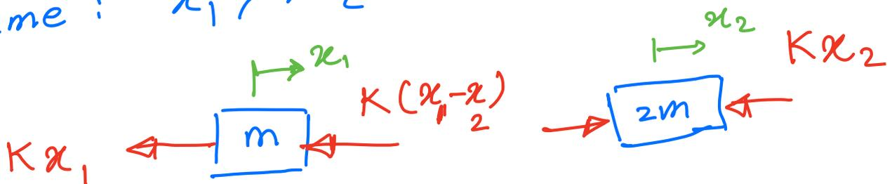
$$\begin{cases} \overset{+}{\rightarrow} \Sigma F = m \ddot{x}_1 & \Rightarrow -Kx_1 - K(x_1 - x_2) = m \ddot{x}_1 \\ \overset{+}{\rightarrow} \Sigma F = 2m \ddot{x}_2 & \Rightarrow K(x_1 - x_2) - Kx_2 = 2m \ddot{x}_2 \end{cases}$$
