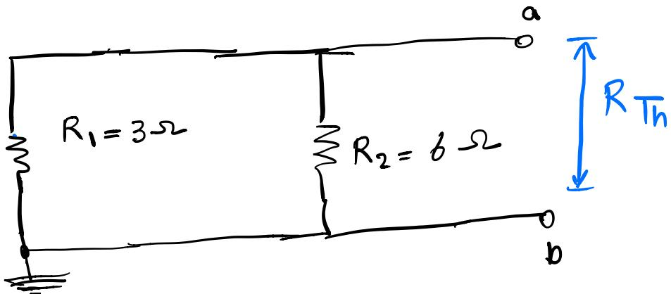
$$R_{Th} = R_1 \parallel R_2 = \frac{(3\ \Omega)(6\ \Omega)}{(3\ \Omega) + (6\ \Omega)} = 2\ \Omega$$
