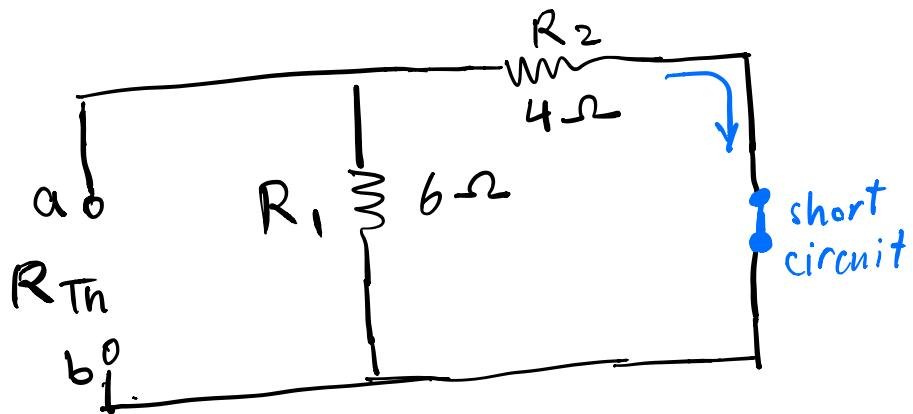
$$R_{Th} = R_1 \parallel R_2 = \frac{(6\Omega)(4\Omega)}{6\Omega + 4\Omega} = \frac{24\Omega}{10} = 2.4\Omega$$
