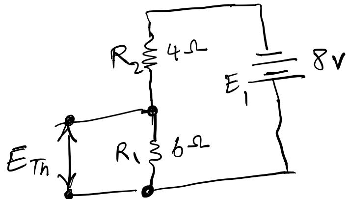
$$E_{Th} = \frac{(6\Omega)(8V)}{6\Omega + 4\Omega} = \frac{48V}{10} = 4.8V$$
