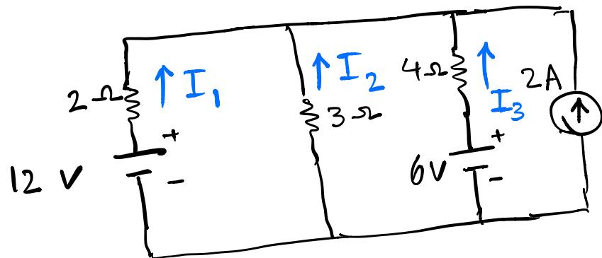
To Find  $R_{Th}$ , disconnect the  $3\Omega$ , short circuit voltage sources and open circuit current sources as shown.
