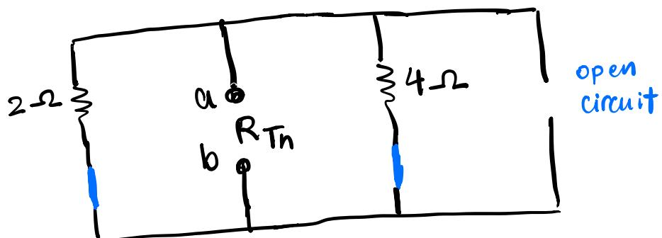
$R_{Th}$  is the total resistance of the circuit between a and b. In this case the  $2\Omega$  and  $4\Omega$  resistors are connected in parallel and
