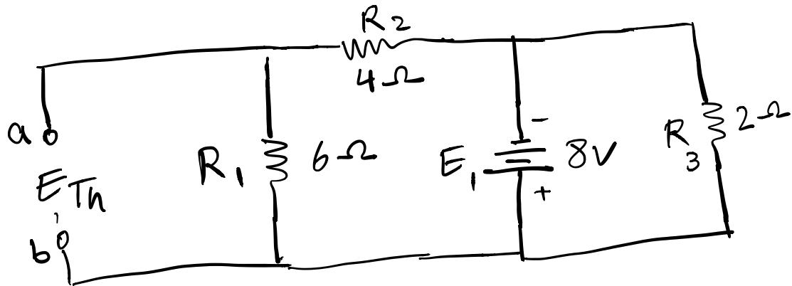
The voltage is the same across parallel elements. Therefore, the voltage across  $R_1$  is  $E_{Th}$  and  $R_3$  is 8V.
