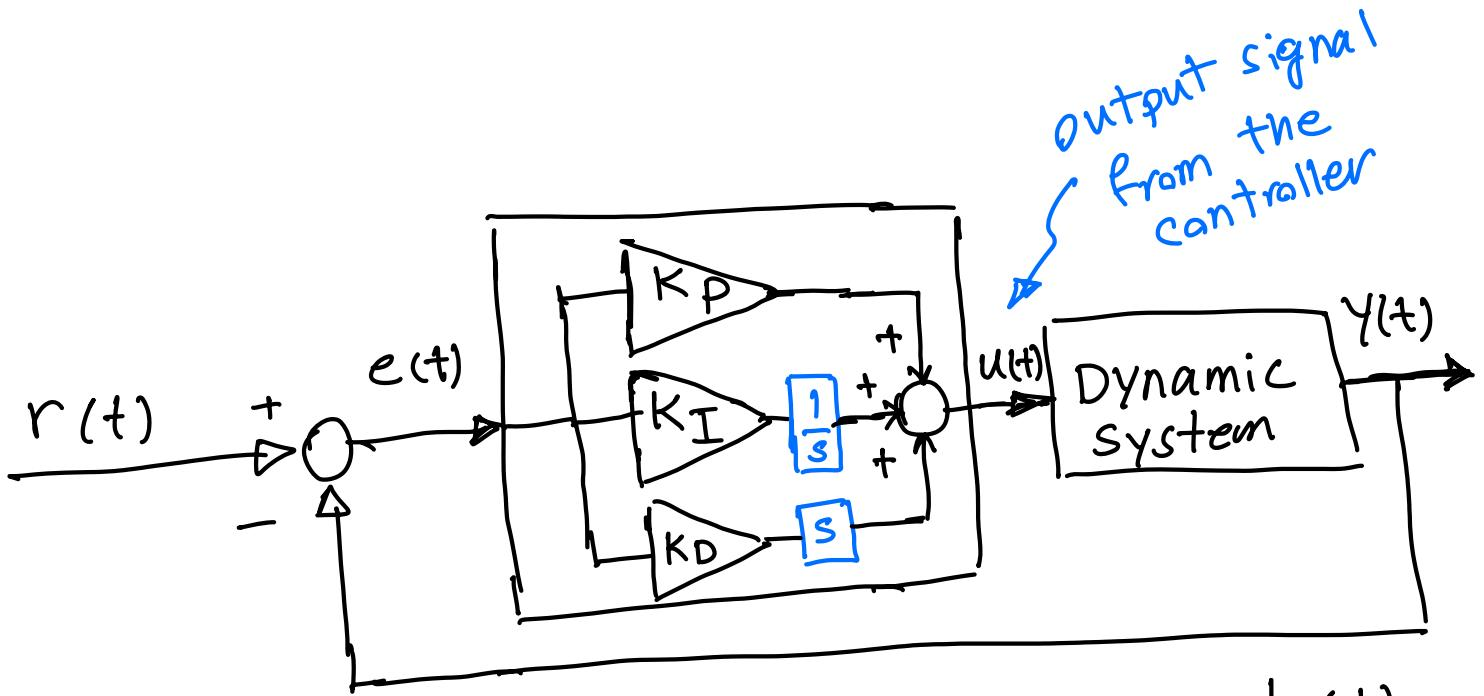
$$u(t) = \underbrace{K_P e(t)}_{\text{proportional controller with proportional gain of } K_P} + \underbrace{K_I \int e(t) dt}_{\text{Integral controller with the gain of } K_I} + \underbrace{K_D \frac{de(t)}{dt}}_{\text{Derivative controller with the gain of } K_D}$$
