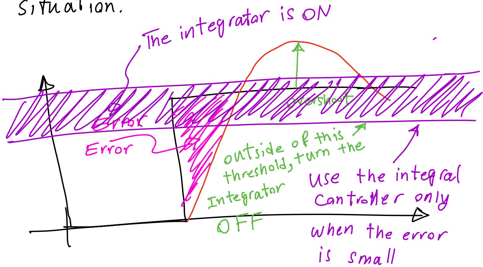
Therefore, turn on the integrator using a switch only when the error is small, and turn off the integrator for other error values.
