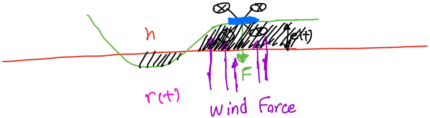
As the drone moves the integral controller adds the area under the error curve to the control signal. Therefore, the control signal becomes larger and larger until the drone force due to the larger control signal becomes larger than the wind force.
