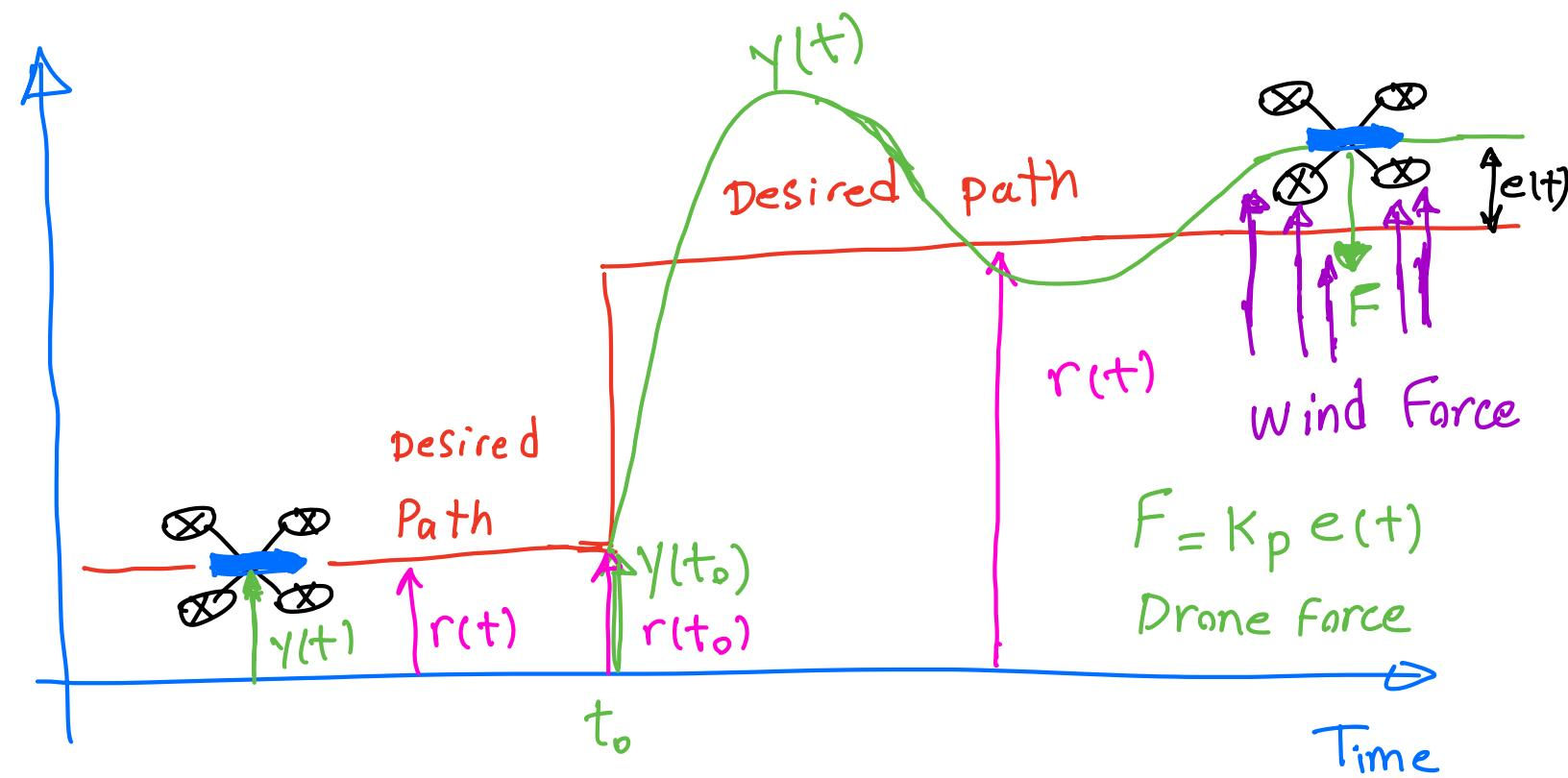
The wind force is pushing the vehicle away from the desired path. Also, the error can be small.
