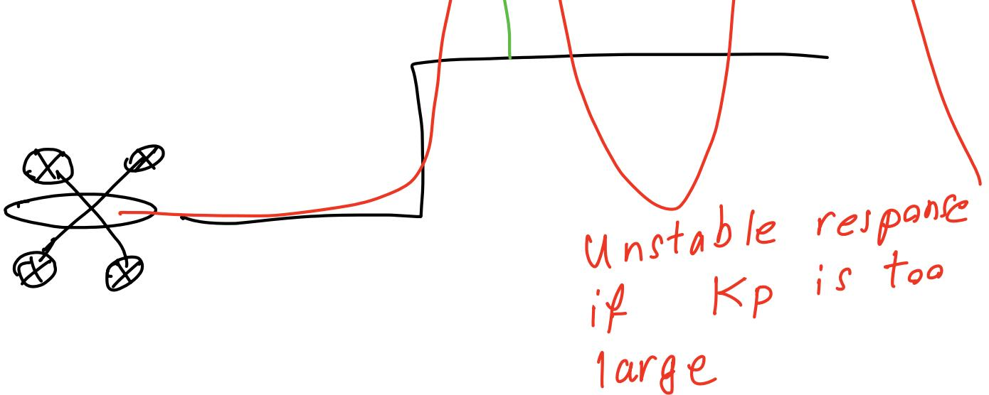
The derivative controller reduces overshoot and allows to increase  $K_p$  without making the system unstable.
